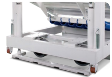
Dynamic Sub Frame in game position (down). Steel bar with resilient protective pad evenly distributes weight, helps protect floors and absorbs the impact of slam dunks.
