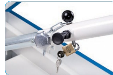
Automatic snap lock on telescopic rod. Locking pin secured with deadlock.
